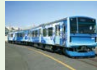
HYBARI hydrogen hybrid train Photo: East Japan Railway Company
